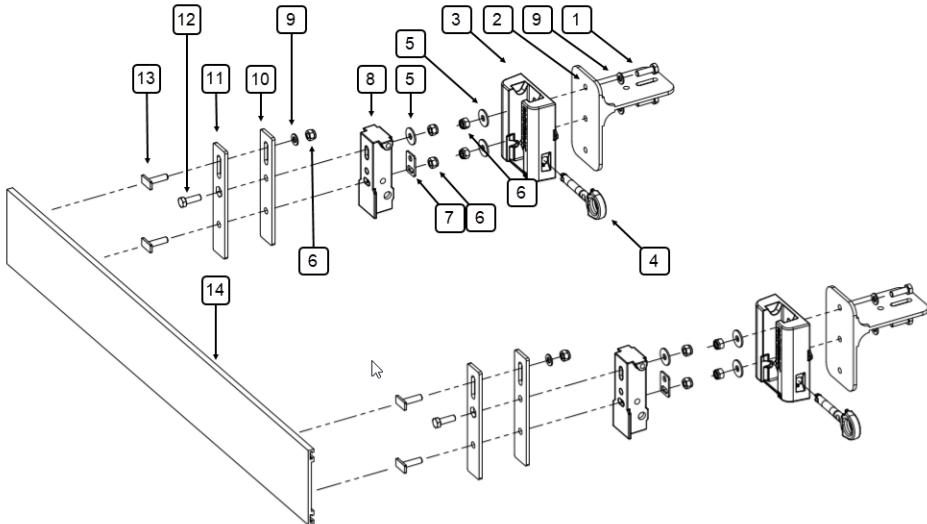
1. M8 x 20mm bolt (supplied with the RacksBrax HD Hitch Standard)
